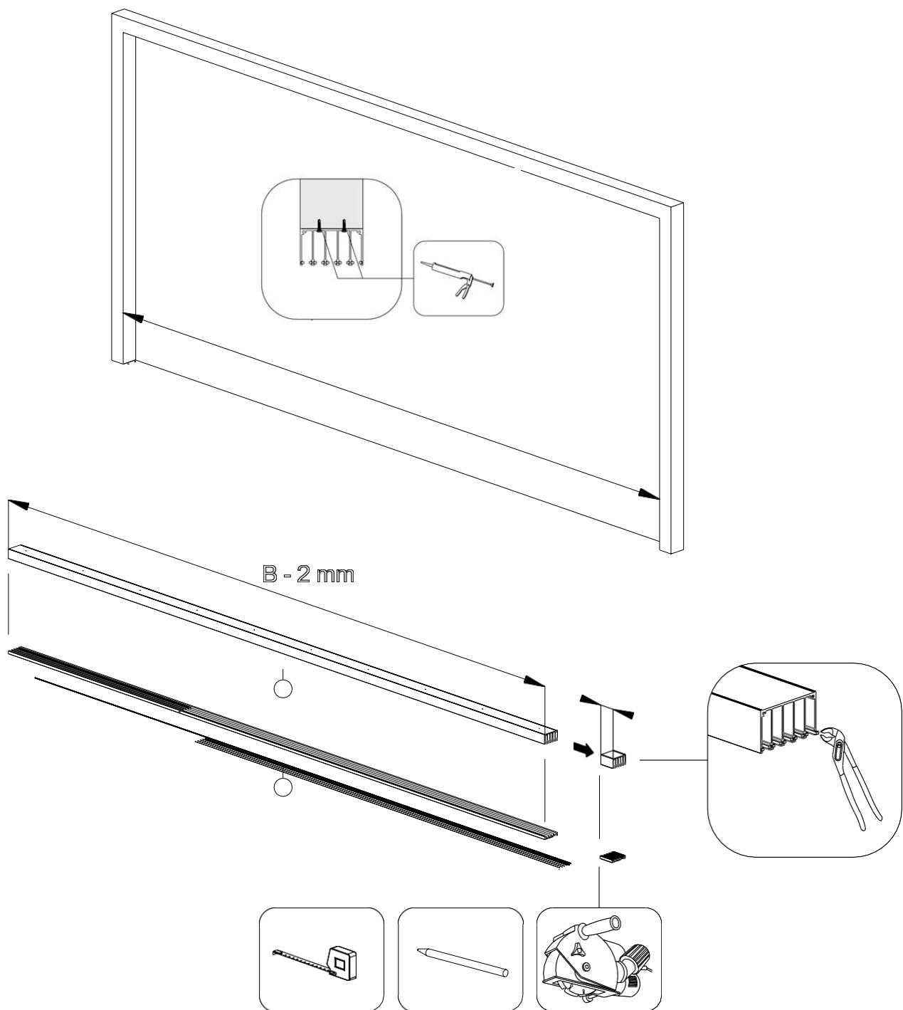
**EN:** Slide the rubber strip onto the glass and then tap the aluminium profile over it.
