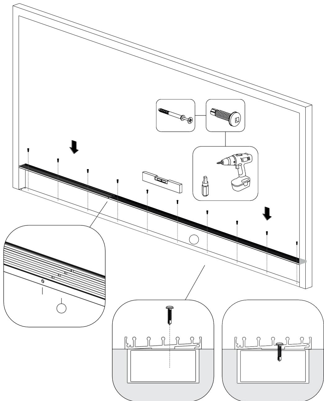
**EN:** Now measure the total height and cut the u-profiles (side profiles) to this. Then screw these into the construction.
