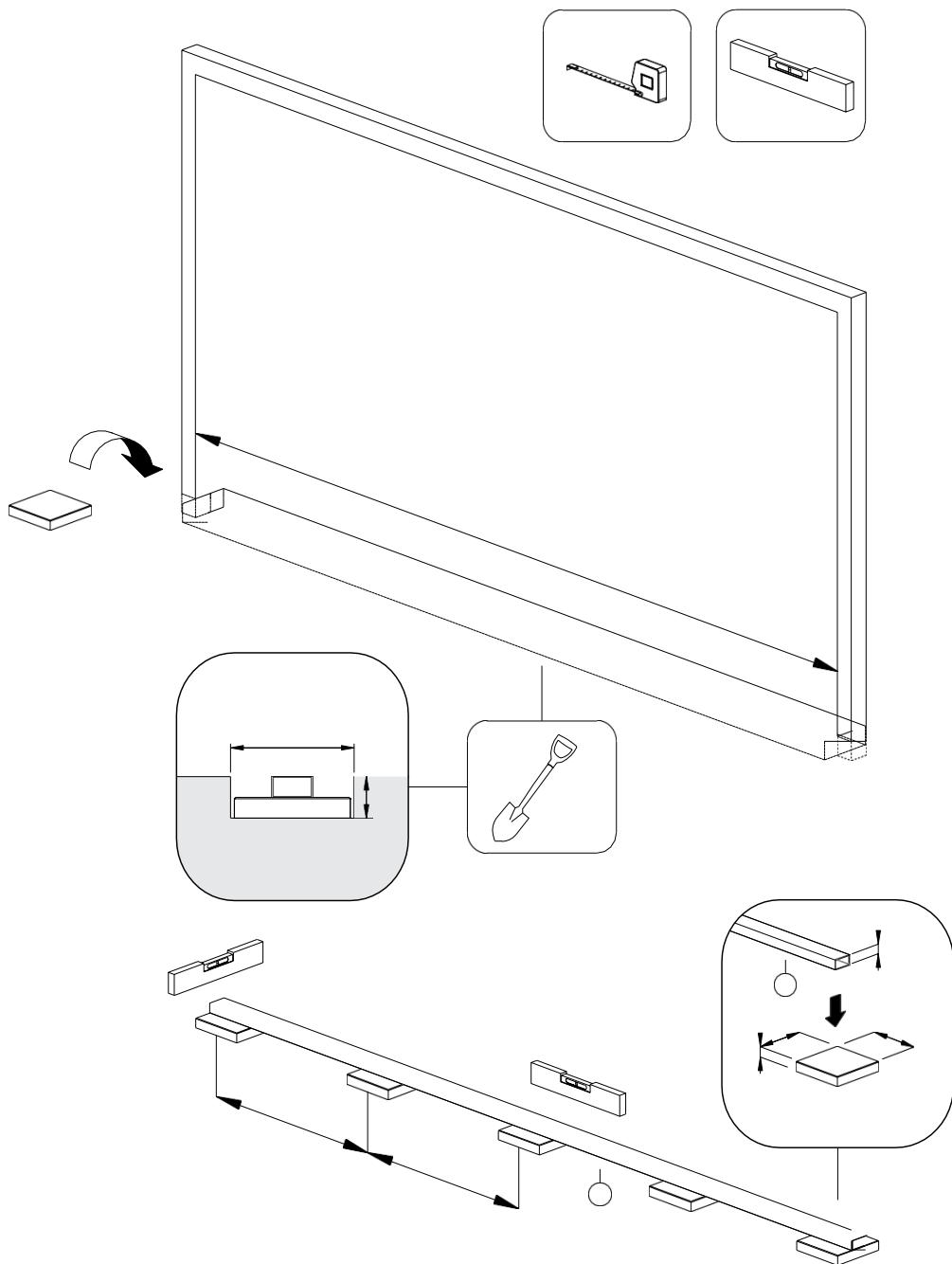
**EN:** Cut the foundation tube 2 MM smaller than the desired size.
