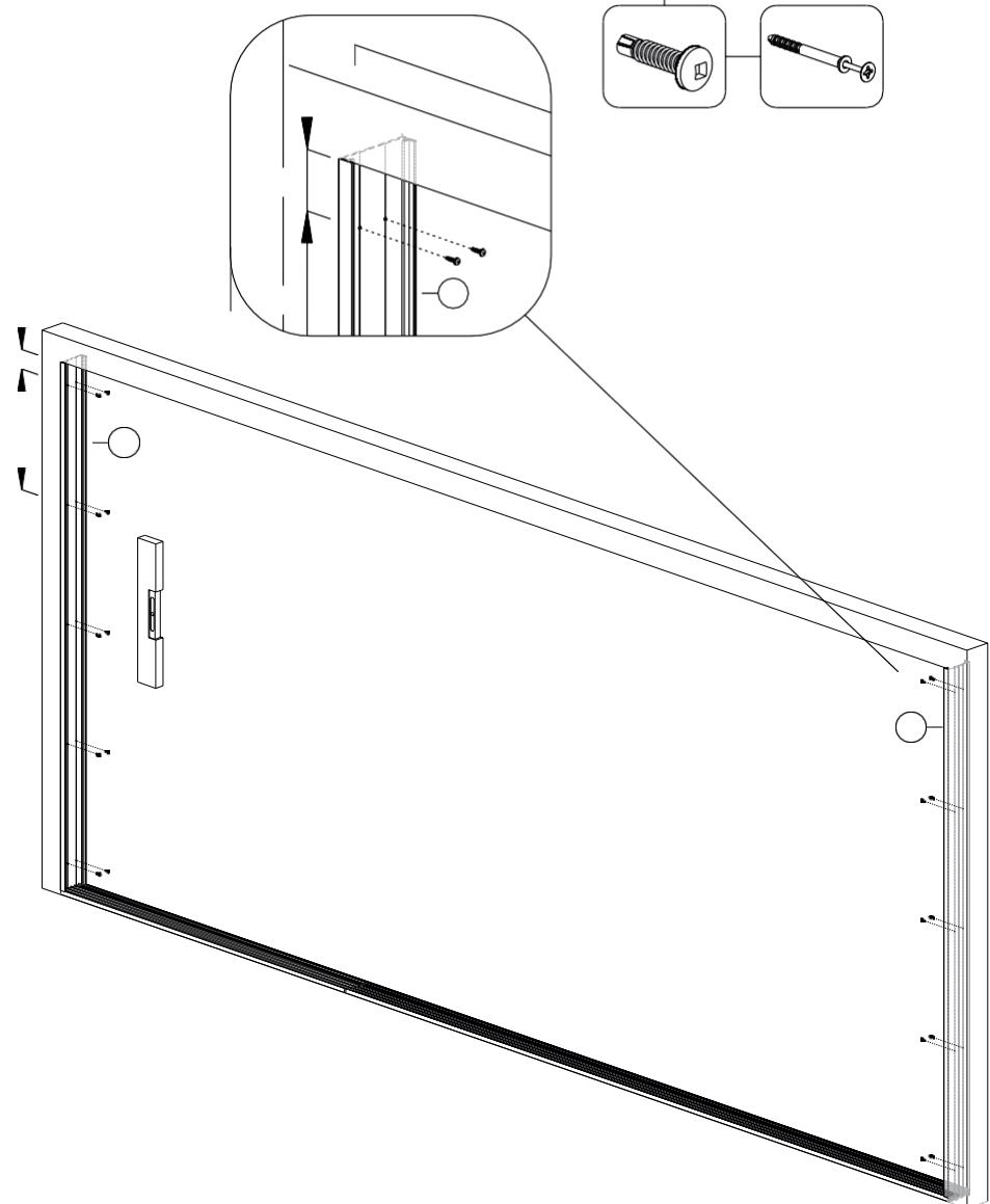
**EN:** First slide the draught strips into the profile, then squeeze the profile slightly with pliers (see illustration). Cut the top and bottom rail 2 MM smaller than the desired size and screw it to the top of the canopy.
